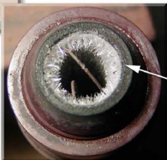
Fig 8.14.13 - These images show the interior of our quartz autoclave reactor after runs that produced geode-like results. The top-left image shows the female end cap with a dome shaped array of quartz crystals that was discovered when the reactor was opened. The two center images are of the open pipe part of the autoclave after two different runs, showing different crystal structures that grew on the inside of the pipe. The large crystal wrapped in wire was covered with tiny quartz crystals, a surprise since this had not happened during previous quartz growth experiments. What caused this nucleation of small crystals to grow throughout the inside of the autoclave? The only thing that changed was the addition of wood. These man-made geodes are the result of wood petrification experiments inside the autoclave. The disintegration of the wood in the reactor created tiny seeds that stimulated the precipitation of the quartz in solution, causing a remarkable crystallization event. More details about these experiments will be discussed in the upcoming Fossil Model Chapter.
