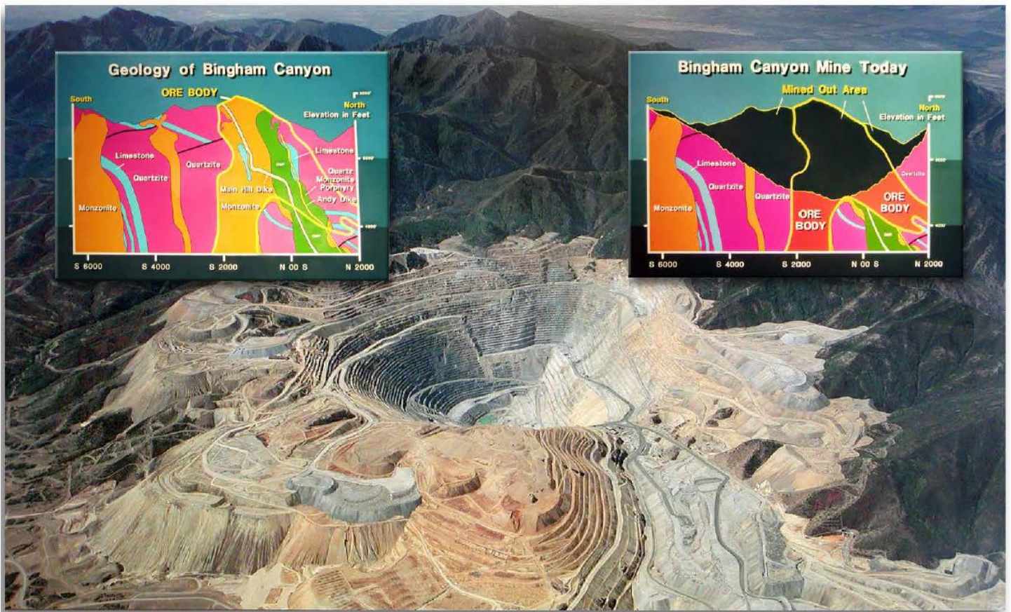
Fig 6.8.3 – This is the Kennecott Copper Mine as seen from the air. Quite literally, an entire mountain has been removed. The insets are cross-cut diagrams illustrating a vertical view of the ore layers—before mining on the left, today on the right. Notice the ore bodies are in vertical or near-vertical orientation, showing they had to have formed from rising material. If this material was not magma, what was it? How did ore bodies like these really form?
