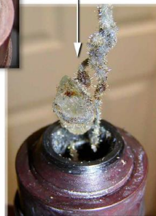
Fig 8.14.13 - These images show the interior of our quartz autoclave reactor after runs that produced geode-like results. The top-left image shows the female end cap with a dome shaped array of quartz crystals that was discovered when the reactor was opened. The two center images are of the open pipe part of the autoclave after two different runs, showing different crystal structures that grew on the inside of the pipe. The large crystal wrapped in wire was covered with tiny quartz crystals, a surprise since this had not happened during previous quartz growth experiments. What caused this nucleation of small crystals to grow throughout the inside of the autoclave? The only thing that changed was the addition of wood. These man-made geodes are the result of wood petrification experiments inside the autoclave. The disintegration of the wood in the reactor created tiny seeds that stimulated the precipitation of the quartz in solution, causing a remarkable crystallization event. More details about these experiments will be discussed in the upcoming Fossil Model Chapter.
