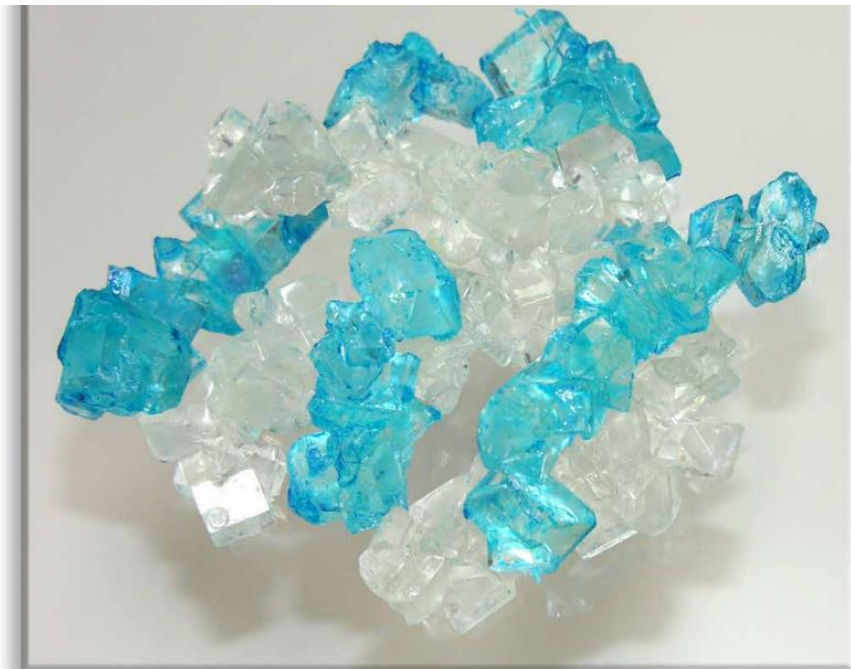
Fig 7.4.2 – These are sugar crystals formed on strings suspended in super-saturated sugar water. As water is heated, sugar will dissolve more readily into solution until it becomes ‘supersaturated.’ As the high-temperature, saturated-sugar solution is cooled, sugar crystals precipitate out of the water onto the strings. Blue dye provides added color. This is the process for making this tasty ‘rock candy’ treat. It is essentially by the same process that massive, natural salt formations are formed.
