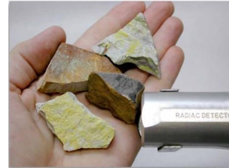
Fig 5.6.1 – 'Hot' radioactive uranium ore sets a Geiger counter buzzing, but is no hotter (temperature wise) than any other rock
