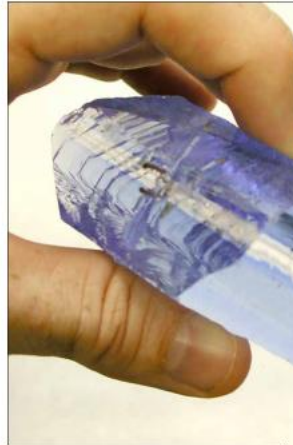
Fig 7.4.14 – This is a man-made quartz crystal grown for technological purposes. The clear strip seen in the bottom photo is the quartz 'seed' while the blue material is the grown quartz. The addition of the element chromium is responsible for the blue color.
