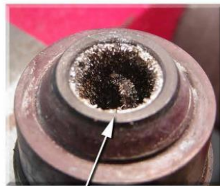
Male end of the reactor shows different runs with crystals growing inside of the pipe.
