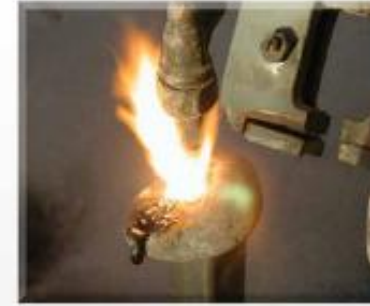
MELTING ROCK WITH TORCH
