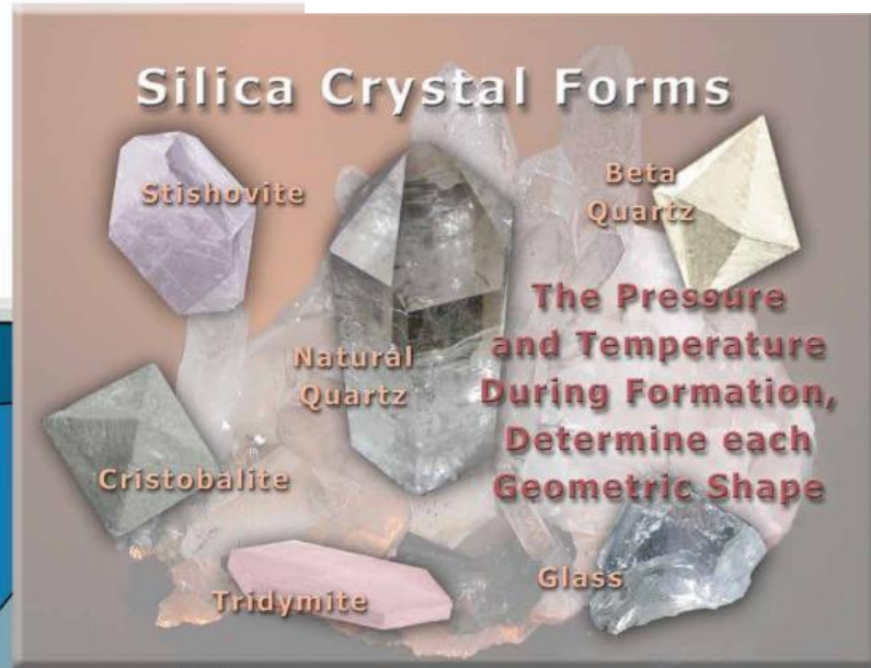
Fig 7.4.17 - Silica or SiO 2 , can occur in various crystalline forms affected by heat and pressure. While Natural Quartz (alpha-quartz) occupies only a small segment of the diagram, Natural Quartz, being formed at the lowest temperatures and pressures, makes up 99.999% of SiO 2 minerals. Other high pressure or high temperature crystalline forms make up less than .001% of SiO 2 rocks.
