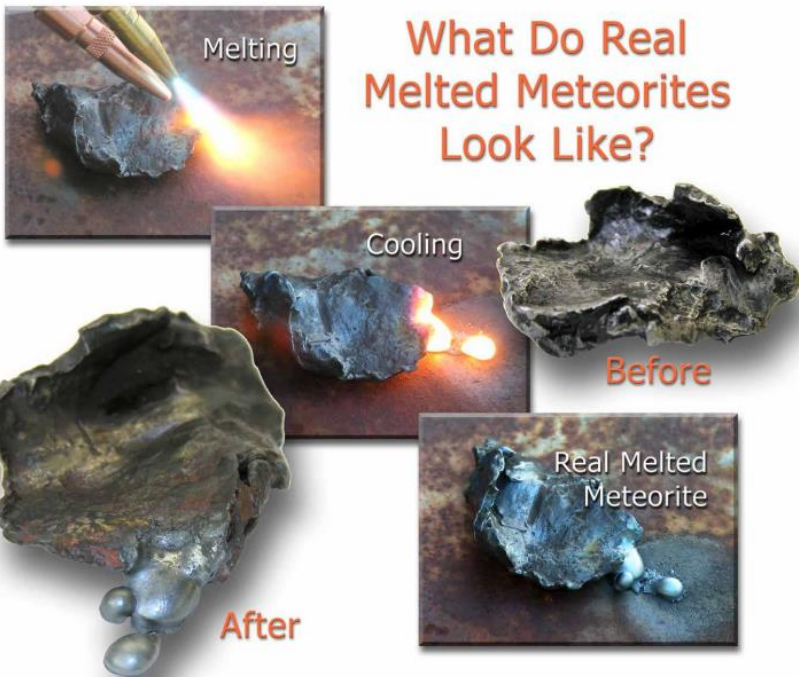
Fig 7.10.7 – This simple melting exercise demonstrates one reason why meteorites did not come from a magmaplanet core. It also shows what meteorites melted during an impact would really look like. Anyone with welding experience can relate to the iron 'beads' that form from melted iron and melted iron meteorites are the same. This photo group includes before and after images of a piece of the Sikhote-Alin meteorite. The melted metal takes on a completely different appearance. The widely accepted origin of meteorites attributes them to the asteroid belt, which is assumed to be the remnant of a magmaplanet core. Most meteorites show no evidence of melting, whether by impact or by being a magmaplanet core remnant.
