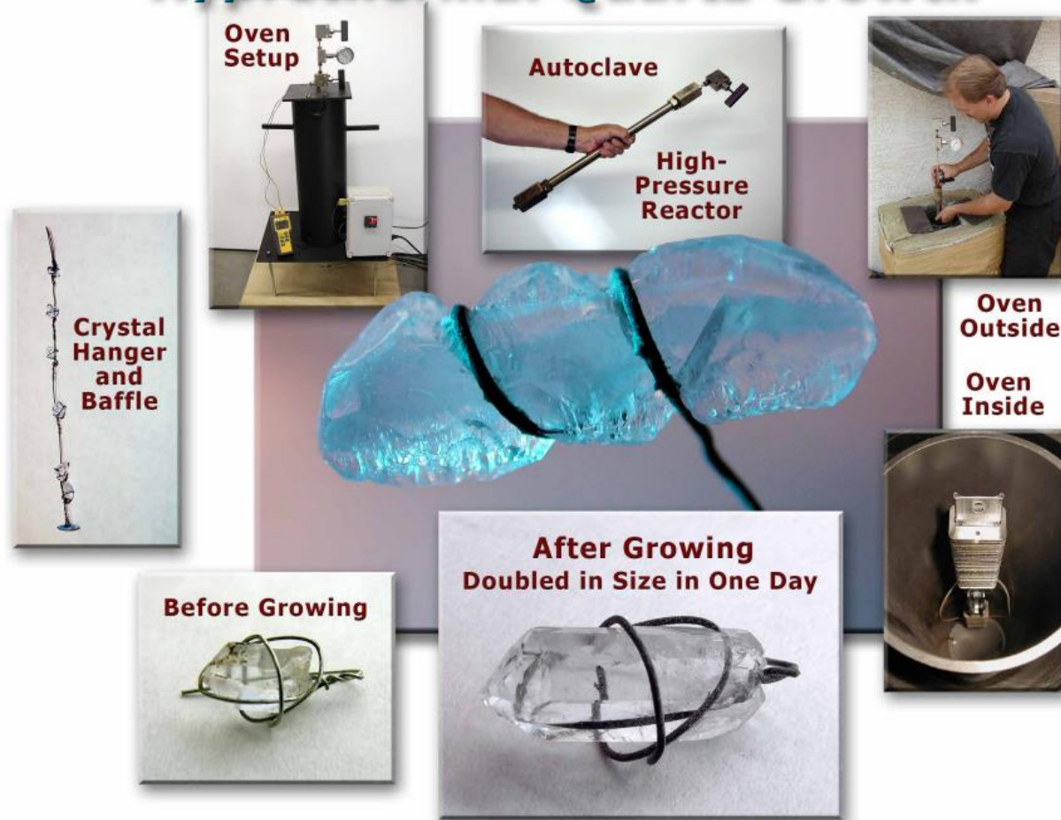
Fig 7.4.13 – This diagram illustrates the hyprethermal quartz-growth process. The word hyprethermal is a merger of the words "hydro" (water), "pre" (pressure), and "thermal" (heat). A combination of these three physical properties creates a pressurized thermal environment in which quartz crystals can grow. In this diagram, a hanger holding quartz crystal seeds is placed in the high-pressure reactor. A water solution is added to the reactor and it is placed in an oven and heated until the solution reaches 350-400° C. Compare the images of the crystal before growing and after growing. The crystals experienced a rapid growth rate approximately doubling in size in one day , not over millions or even thousands of years.
