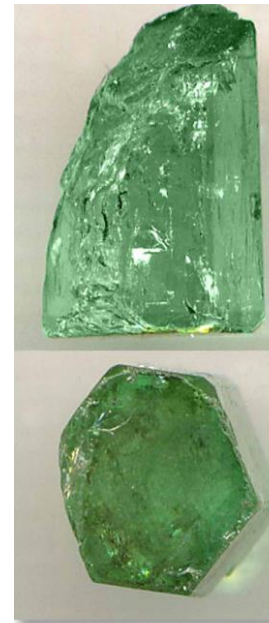
Fig 7.4.16 – Flux-grown (melt) synthetic emeralds have no water in their crystal matrix, whereas all natural emeralds do. Natural emeralds grow in the same manner as quartz but higher pressures and temperatures.
