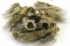
Fig. 5.7.5 – Natural glass tubes known as fulgurites form when lightning strikes and melts sand. Neither natural nor synthetic glass can grow into crystals like natural quartz.
