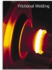
Fig. 5.3.6 - Modern frictional welding with dissimilar metals with frictional heating in a fraction of a second. Courtesy of American Institute of Physics.
