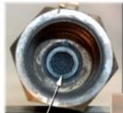
Top female end of reactor shows quartz crystals growing in a dome shape.
