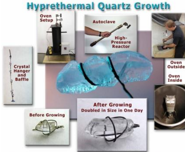
Fig 7.4.13 - This diagram illustrates the hyperthermal quartz-growth process. The word hyperthermal is a merger of the words "hydro" (water), "pre" (pressure), and "thermal" (heat). A combination of these three physical properties creates a pressurized thermal environment in which quartz crystals can grow. In this diagram, a hanger holding quartz crystal seeds is placed in the high-pressure reactor. A water solution is added to the reactor and it is placed in an oven and heated until the solution reaches 350-400° C. Compare the images of the crystal before growing and after growing. The crystals experienced a rapid growth rate approximately doubling in size in one day , not over millions or even thousands of years.
