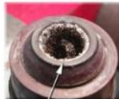
Male end of the reactor shows different runs with crystals growing inside of the pipe.
