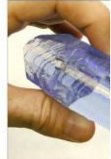
Fig 7.4.14 - This is a man-made quartz crystal grown for technological purposes. The clear strip seen in the bottom photo is the quartz 'seed' while the blue material is the grown quartz. The addition of the element chromium is responsible for the blue color.
