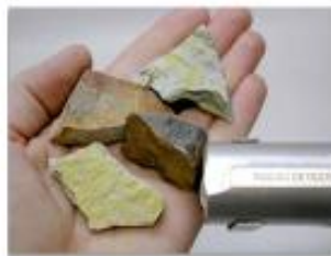
Fig 5.6.1 - "Hot" radioactive uranium ore sets a Geiger counter beeping, but it is no hotter (temperature wise) than any other rock.
