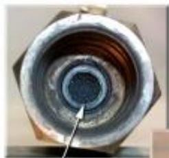
Top female end of reactor shows quartz crystals growing in a dome shape.
