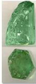
Fig 7.16 - Flux-grown (left) synthetic emeralds have no water in their crystal matrix, whereas all natural emeralds do. Natural emeralds grow in the same manner as quartz but higher pressures and temperatures.
