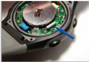
Fig 5.8.2 - The blue arrow is pointing at the quartz oscillator in a quartz watch, which uses the piezoelectric effect to keep time.
