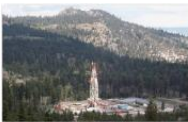
Fig 5.11.1 The Long Valley California, USA, borehole. An attempt to reach a magma body and exploit the heat of magma for energy production failed. No magma was found.
