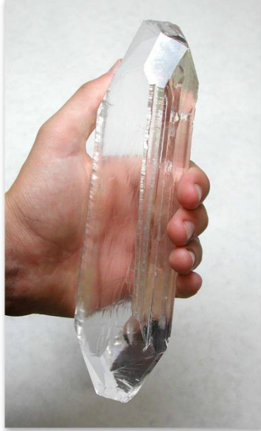
Fig 5.7.1 – This man-made synthetic quartz crystal has the same properties as natural quartz; neither (natural nor man-made) is grown from a melt.
