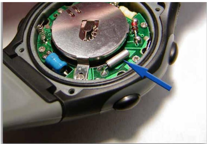
Fig 5.8.2 – The blue arrow is pointing at the quartz oscillator in a quartz watch, which uses the piezoelectric effect to keep time. p.107
