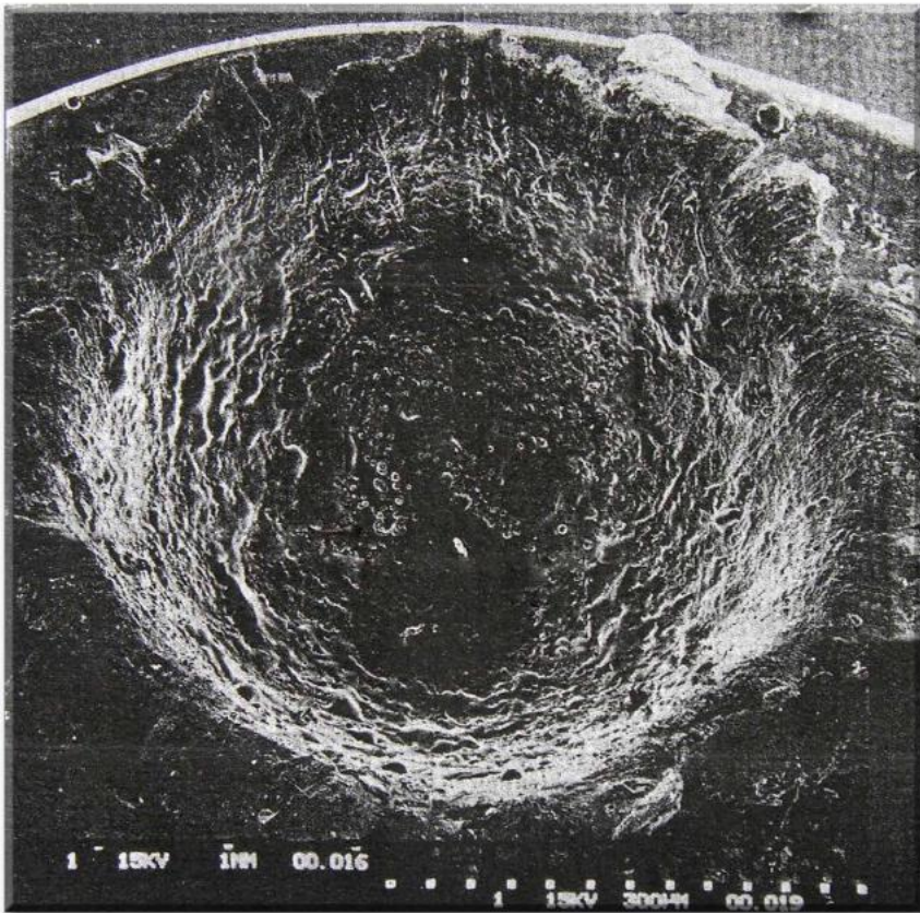
Fig 7.9.11 – A basalt-glass projectile with a velocity of 5.4 km/sec formed this 6.1 mm crater in aluminum. The experimenters described the crater: “Note that the entire crater is relatively evenly lined with projectile melt ”. The researchers go on to say that the melt is, “ easily recognized even by the naked eye ”. This photo is from the second of five journal articles describing hypervelocity melt.
