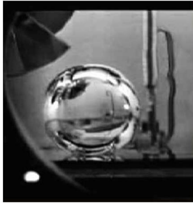
Fig 7.1.2 – This sphere is a large air bubble formed on a hotplate, underwater in a micro-gravity environment, in orbit above the Earth. It illustrates how spherical shapes form when the forces of gravity are neutralized. This applies to both liquids and gases. Courtesy of NASA. p.232
