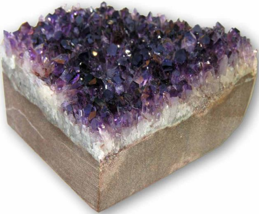
Fig 7.4.15 – This is a cross section showing natural quartz (white) on a sandstone base with synthetic amethyst quartz (purple) grown on top of the natural quartz. This specimen was made in Russia where much research involving the use of autoclaves was conducted, prior to the collapse of the Soviet Union. This specimen helps illustrate how natural quartz grows in a hypretherm.
